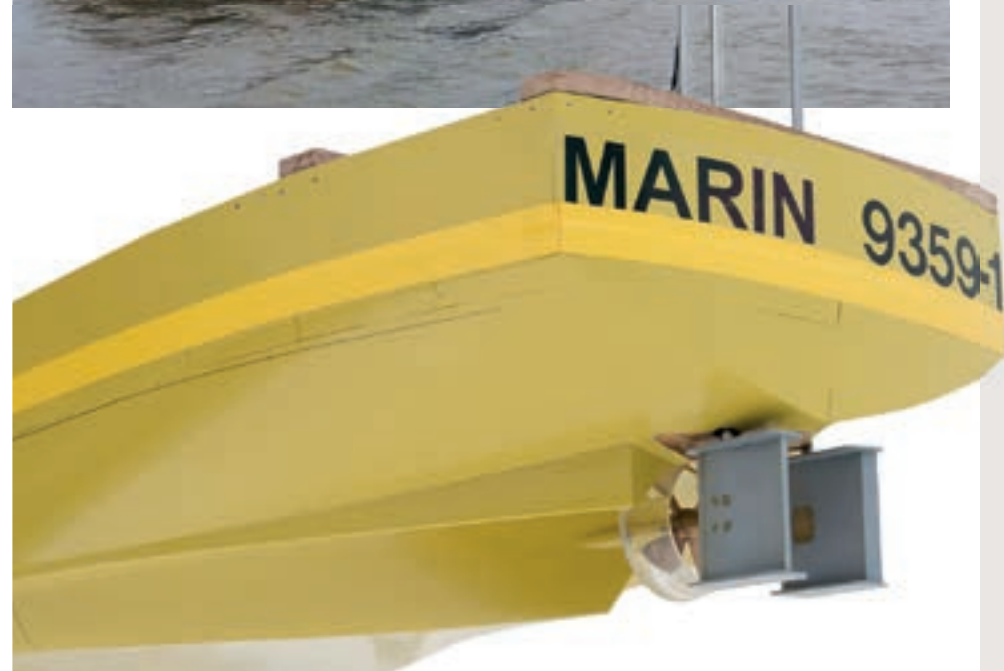
Ship model used to test different rudder configurations
